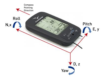
Figure 8.2: Compass Calibration Reference Frame
